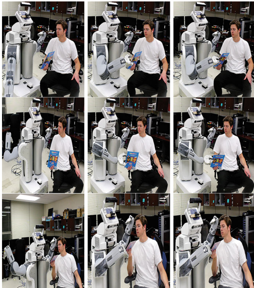
Fig. 12 Robot grasping an object held by a human. Left: initial position of the robot's gripper, middle: gripper adapting to the object's pose, right: grasping of the object
