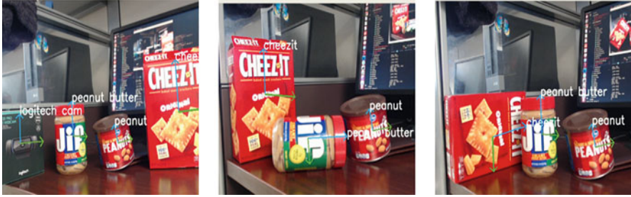
Fig. 9 Multiple object detection with estimated planar vectors
