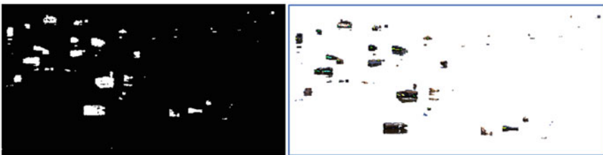
Fig. 6 (Left) Mask for the floating surface debris of Fig. 1b. (Right) Extracted debris from the original image (Fig. 1b) using the debris mask with white background for enhanced contrast
