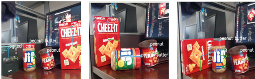
Fig. 9 Multiple object detection with estimated planar vectors
