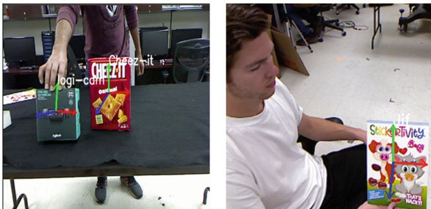
Fig. 10 (a) Pose estimation of multiple objects (b) Estimated pose of an object held by a human
