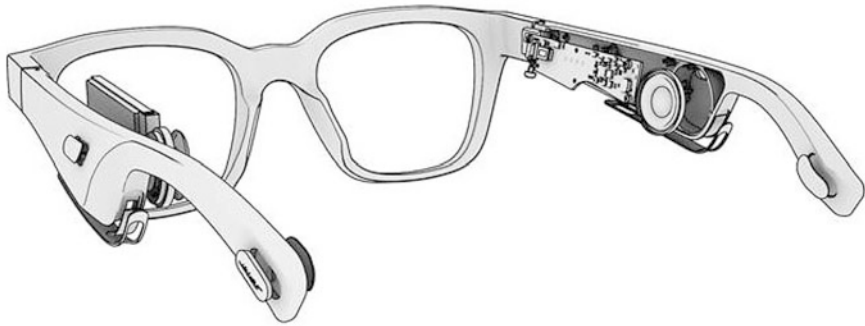
Fig. 1 The wearable sensor used in this study to perform activity detection. Picture courtesy of Bose
