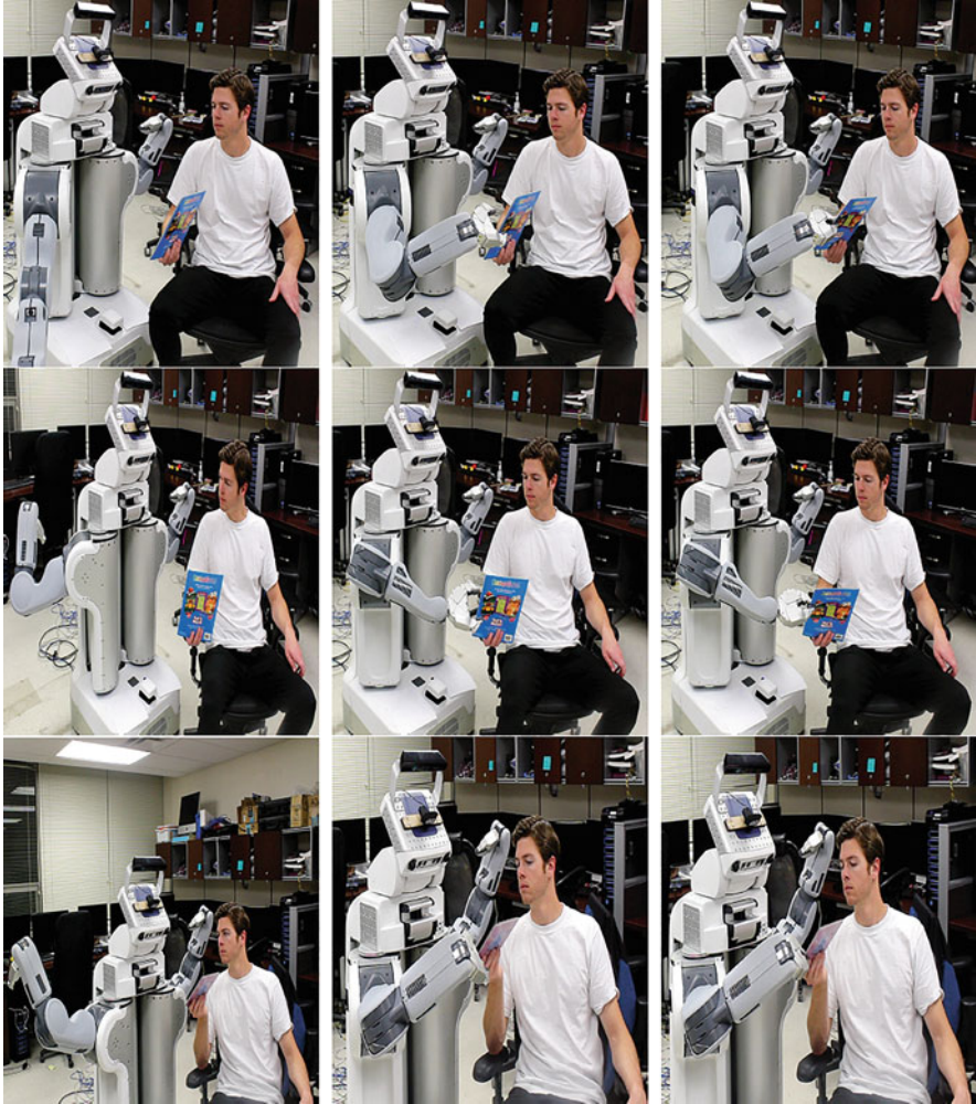
Fig. 12 Robot grasping an object held by a human. Left: initial position of the robot's gripper, middle: gripper adapting to the object's pose, right: grasping of the object
