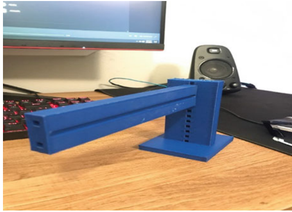
Fig. 9 Disassembled portion of the Mk. 3 chassis support crossbar
