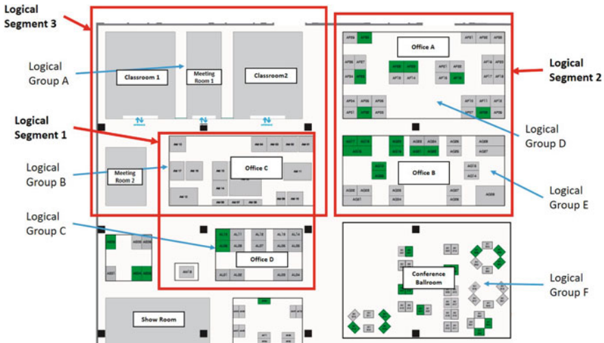
Fig. 2 Concept of the logical segment and logical group in the dynamic clustering method
