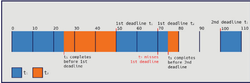
Fig. 3 Worst-case scenario for tasks t_1 and t_2 . Deadlines are missed despite being below processing capacity
