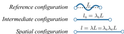
Fig. 5.21 Different configurations during the stretching of an undulated fiber. In the reference configuration, the fiber has the length L , whilst l_s denotes the straightened out but still unstressed fiber
