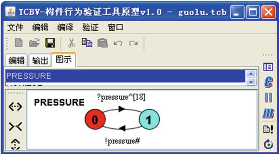
Fig. 1 States migration diagram of pressure sensor's protocol
