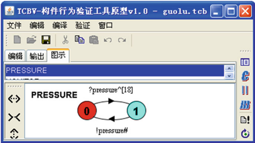
Fig. 1 States migration diagram of pressure sensor's protocol
