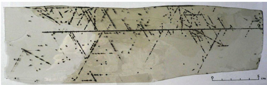
Fig. 6 A sheet of mica muscovite showing a quodon primary track and many secondary tracks scattered from it. Also it is possible to see the intermittency in the secondary tracks along the close packed direction of the cation layer. This is interpreted as a quodon loosing and regaining a positive charge. Reproduced with permission from: Russell and Eilbeck [30]. Copyright © 2011, AIMS
