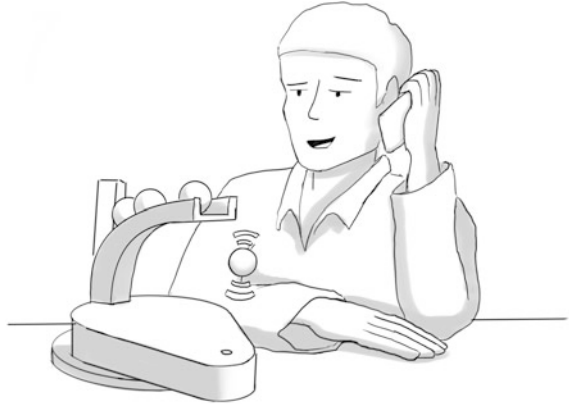
Fig. 7 Artist's drawing of The Hover, a device that augments telecommunication by conveying activity and presence of remote partners
