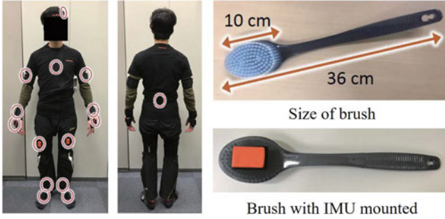
Fig. 20 Mounting positions of the IMU sensors on the user’s body and dimensions of the brush used
