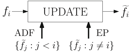
Fig. 3.11 Diagram of ADF and EP updates for a single iteration. The ADF limits itself by looking at the previously included factors, which got approximated from f_j to \tilde{f}_j in the projection step of q^j . The EP considers all factors simultaneously, except for the one to be updated, what avoids factor multiplicity in the approximation q
