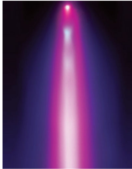
Fig. 9.33 Images of the plasma jets in the LPPS®-TF process, chamber pressure 200 Pa (2 mbar), plasma Jet length 2 m, Jet diameter 200–400 mm, torch power up to 180 kW with 4 powder injectors. [image and info courtesy of Ö relikon-Metco corporation]
