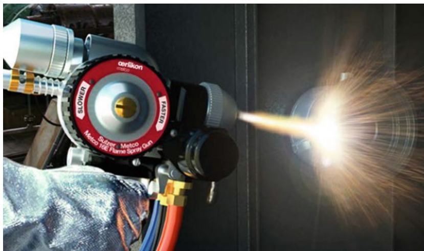
Fig. 7.13 Photograph of the Oerlikon-Metco 16E Wire Flame Spray gun. (Photograph Courtesy of Oerlikon-Metco)
