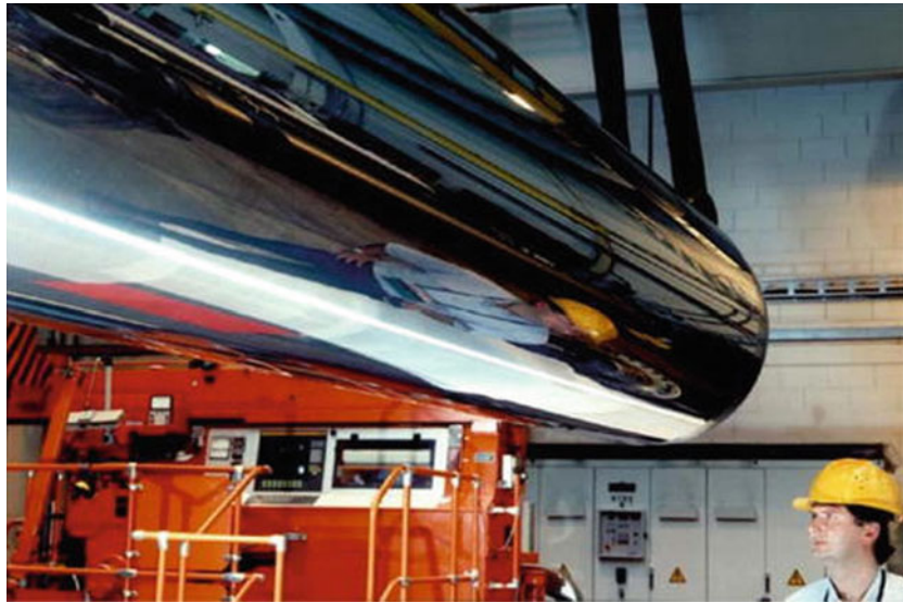
Fig. 19.16 SUME™CAL coating after super-finishing on calendar roll. (Courtesy of Oerlikon-Metco)
