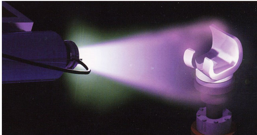
Fig. 19.14 Vacuum plasma spraying of HA coating on a knee prosthesis
