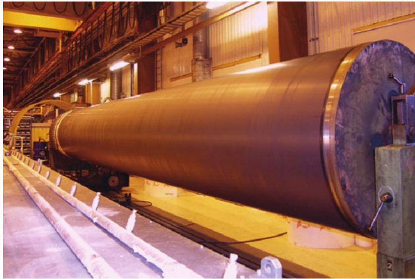
Fig. 19.19 Paper machine center press roll with a thermally sprayed ceramic coating (Metso Paper Inc.). (Reproduced with kind permission from ASM [Vuoristo P, Nylén P (2009)])
