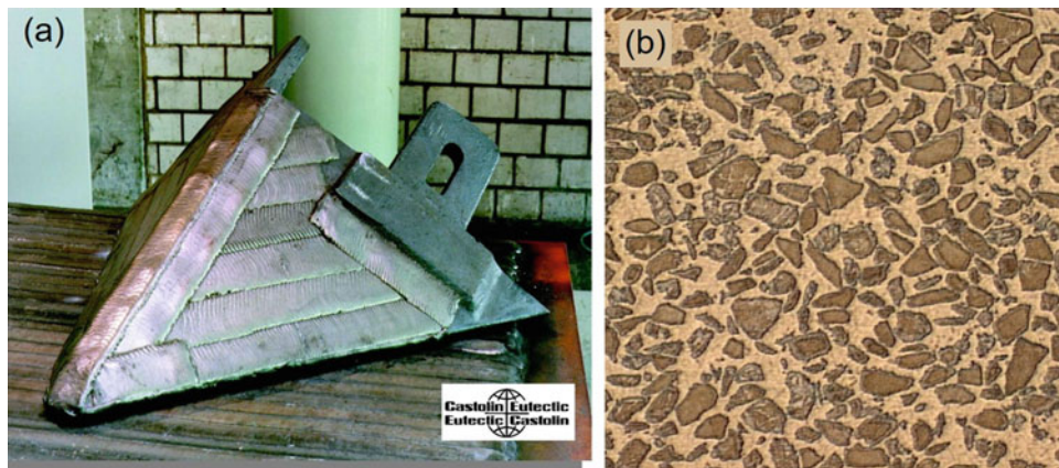
Fig. 19.27 (a) Tooth of excavator PTA-coated with a nickel-based composite (b) coating microstructure. (Courtesy of Castolin)
