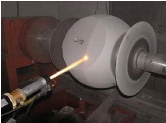
Fig. 19.21 General view of practical spraying of ball valve by the MET-JET III system. (Reprinted with kind permission from ASM [Huang XO, et al. (2007)])
