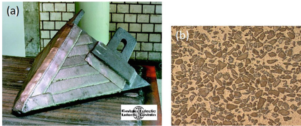
Fig. 12.38 (a) PTA coated tooth of excavator with Ni base coating + WC (25 kg/h). (b) cross section of the coating (courtesy of Castolin)
