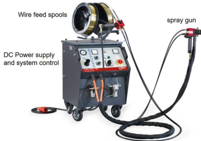
Fig. 11.32 General view of an Oerlikon Metco Flexi Arc™ 300 wire arc spray unit. (Reproduced with kind permission of Oerlikon Metco)
