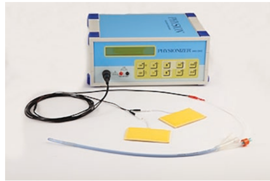
Fig. 11.2 EMDA device and catheter
