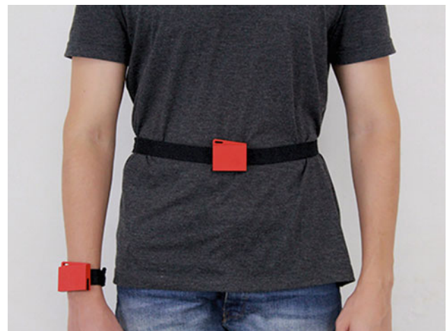
Fig. 2 Body locations where SensorTags were attached: one at the waist and the other at the right wrist
