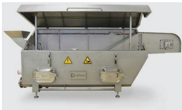
Fig. 4 PEF processing system for solid products with a capacity of 1 to 6 t/h
