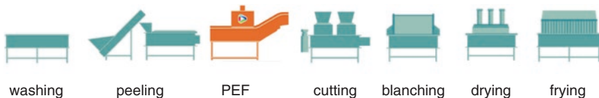
Fig. 1 Industrial French fry processing line including PEF. (Elea GmbH 2020)
