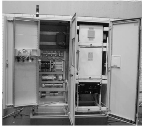
Fig. 41 20 kJ/s/20 kV monopolar solid-state PEF pulser. (Source: AMS Electronics/Propuls)
