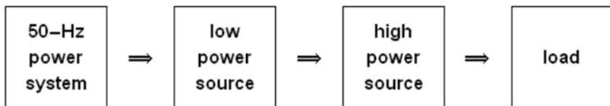
Fig. 8 Basic setup of pulsed power systems for the generation of pulsed electrical fields
