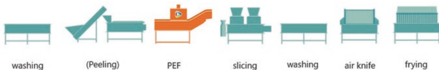
Fig. 5 Industrial potato chips processing line including PEF. (Elea GmbH 2020)
