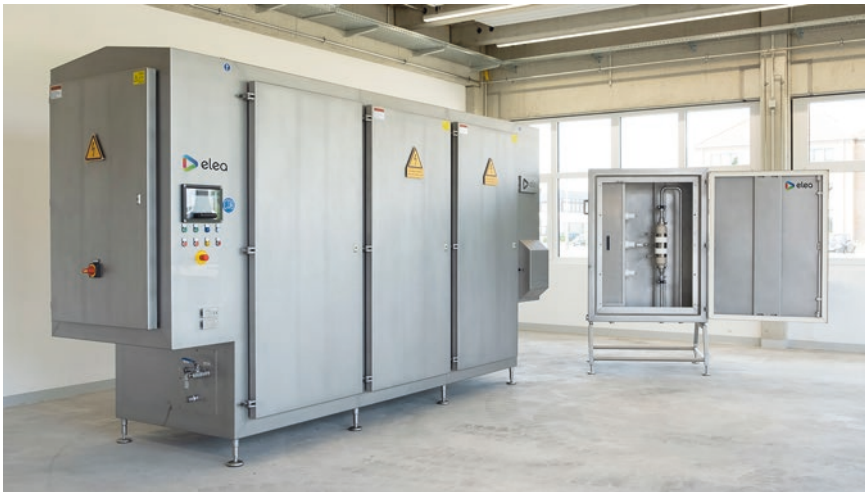
Fig. 1 Industrial-scale system for fruit juice preservation, up to 5.000 l/h
