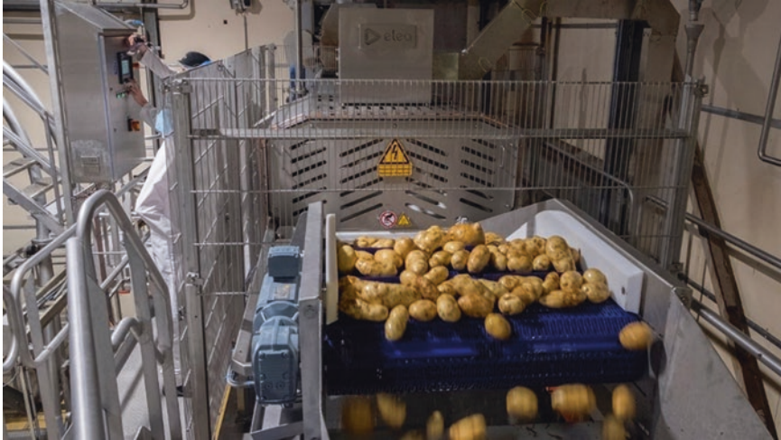
Fig. 2 Potato outlet of an industrial PEF system in a French fry processing line. (Elea GmbH 2020)
