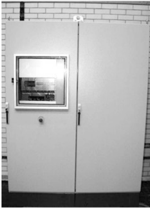
Fig. 41 20 kJ/s/20 kV monopolar solid-state PEF pulser. (Source: AMS Electronics/Propuls)
