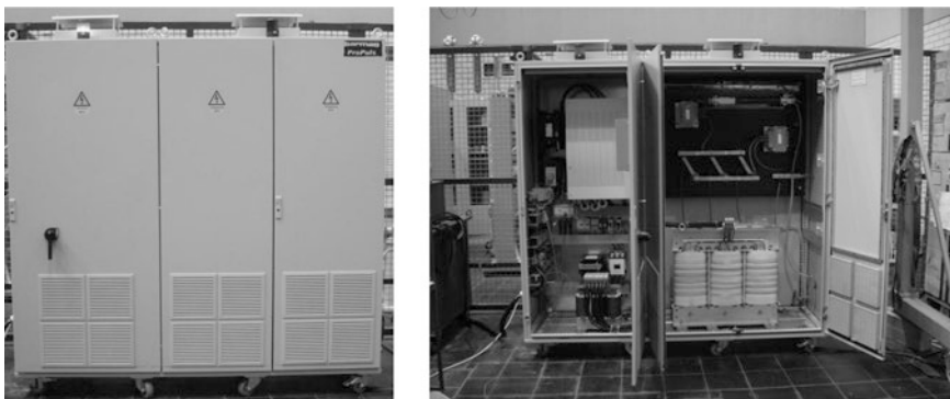
Fig. 40 35 kJ/s/18 kV power supply. (Source: BARMAG, Propuls)
