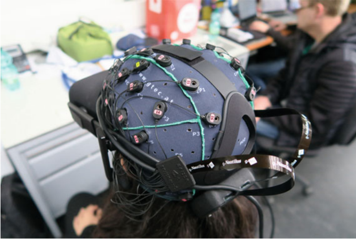
Fig. 9.3 The 32 electrodes EEG device used in COGITO in Space . Photo Sandro Bocci, 2017 (de Paulis 2019, 2021a, b)
