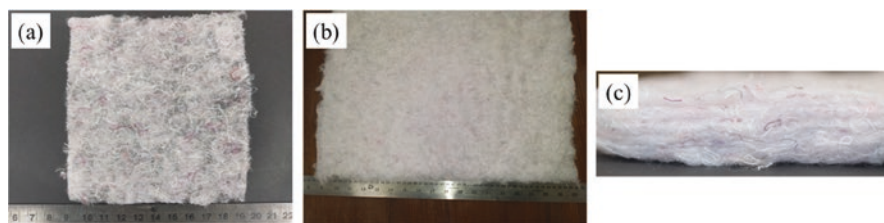
Fig. 2. A piece of a single layer of the fibre web (a), multi-layered carded web (b) and its cross-sectional view (c).
