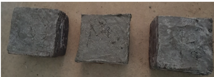
Fig. 1. PET-fibre reinforced concrete after 7 days.
