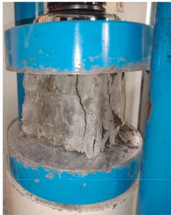
Fig. 8. Compressive strength test on concrete blocks after 7 days.
