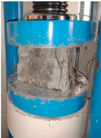
Fig. 8. Compressive strength test on concrete blocks after 7 days.
