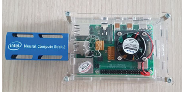
Fig. 2 Raspberry Pi 4 with Intel Neural Compute Stick 2
