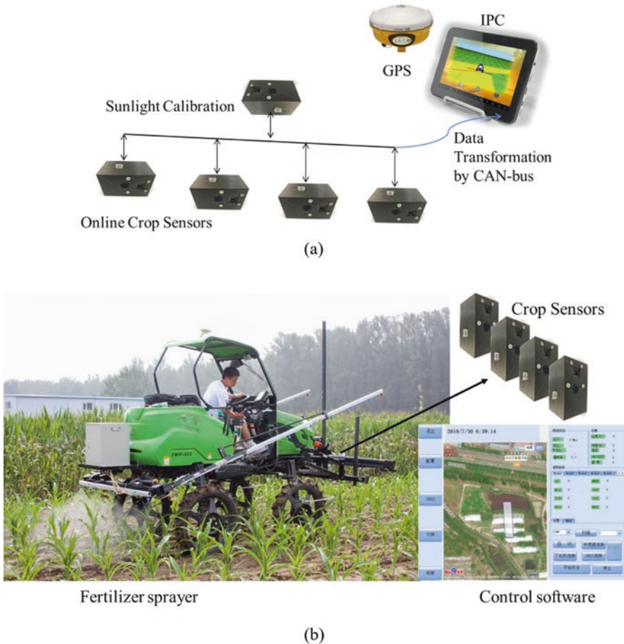
Fig. 8.11 Variable-rate fertilizer control based on crop sensing (a) Sensing system used in a fertilizer sprayer (b) Variable-fertilizer sprayer
