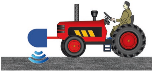
Fig. 4.20 Autonomous measurements of the soil EC based on electromagnetic induction
