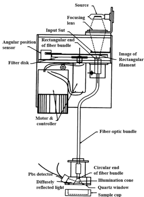
Fig. 3.7 Portable soil sensor. (Sudduth and Hummel 1993)
