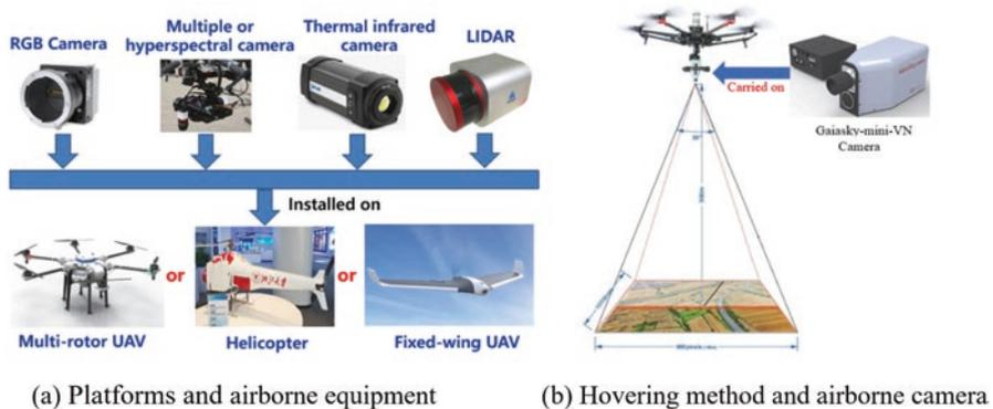
**Fig. 3.10** Remote sensing based on UAVs for soil nutrient detection (a) Platforms and airborne equipment (b) Hovering method and airborne camera
