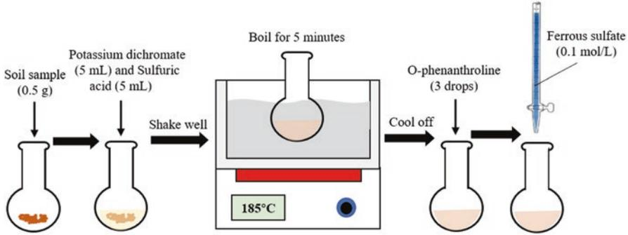
Fig. 3.2 Method of chemical determination for soil organic matter content
