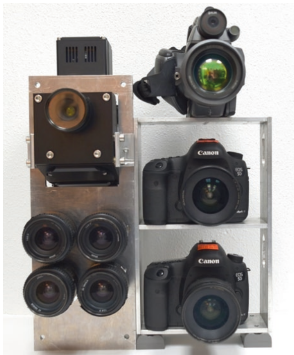
Fig. 6.1 A four-camera imaging system (lower left) mounted along with a hyperspectral camera (upper left), a thermal camera (upper right), and a multispectral imaging system based on two consumer-grade cameras (central to lower right) owned by the USDA-ARS at College Station, Texas
