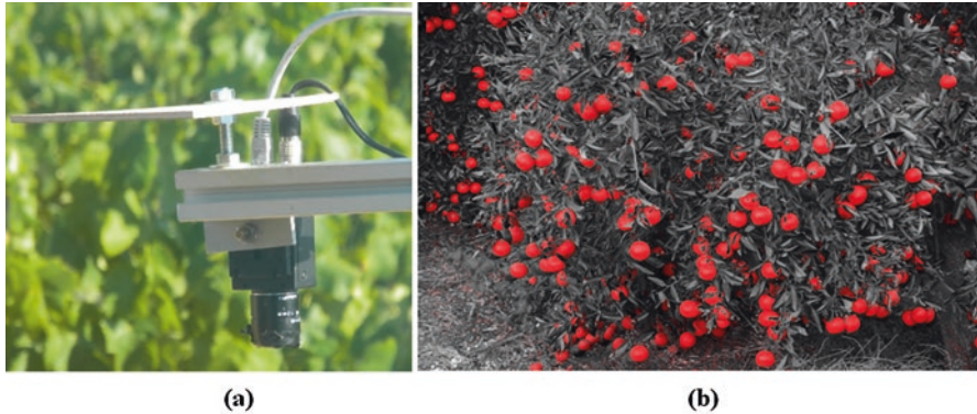
Fig. 5.9 Monocular vision for scouting: (a) digital camera; (b) color image processed to detect oranges
