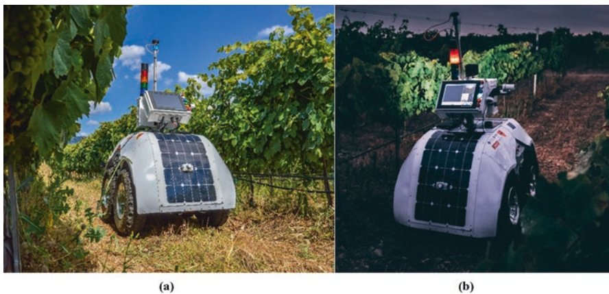
Fig. 5.18 Robot VineScout to assess vine water stress: (a) day mapping; (b) night mapping
