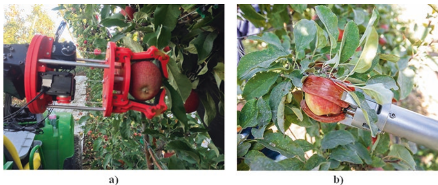
Fig. 8.2 End-effectors with under-actuated fingers designed and developed for picking apples: (a) developed by Silwal et al. (2016); (b) developed by Courtney and Mullinax (2019)
