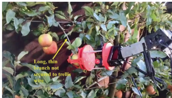
Fig. 16.2 An example of unsuccessful fruit detachment by a robot because of a long and thin offshoot bearing the fruit (from Silwal et al. 2017)
