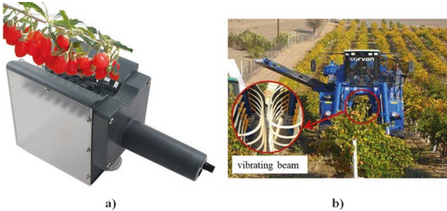
Fig. 8.13 End-effectors designed to directly separate bunches of fruit together: (a) an end-effector developed for wolfberry harvesting with vibration (from Peng et al. 2019); (b) a vibration beam end-effector used to harvest wine grapes (from Huffman 2010)
