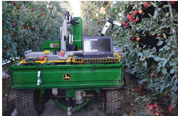
Fig. 7.7 The robotic platform with the arm attached to end-effector, global camera system, and computer during field testing
