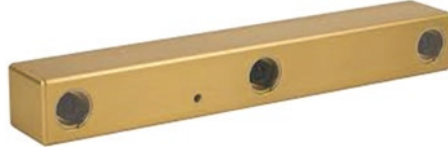
Fig. 3.6 BumbleBee XB3 stereo vision camera from FLIR Systems used in various research projects at Washington State University (e.g., Bhusal et al. 2018; Hohimer et al. 2019; Khanal et al. 2019)
