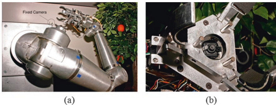
Fig. 9.3 (a) Robotic Research K1207 manipulator with the fixed camera mounted on the stationary base of the robot and (b) the eye-in-hand camera located inside the robot end-effector
