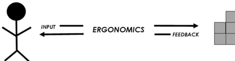
Fig. 15.1 The study of ergonomics is all about the transmission of information that must occur between a machine and its user. Input information is provided to the machine using “controls.” Feedback from the machine is presented to the user through “displays”
