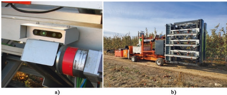
Fig. 3.15 End-to-end system developed for robotic fruit harvesting, conveying, and bin filling; (a) Intel RealSense 435 Cameras used as the color and depth sensors; and (b) the complete harvest system
