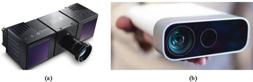
Fig. 3.11 Example 3D Cameras; (a) CamCube 3 from PMD Technologies (Siegen, Germany); and (b) Azure Kinect from Microsoft Inc. (Redmond, WA)
