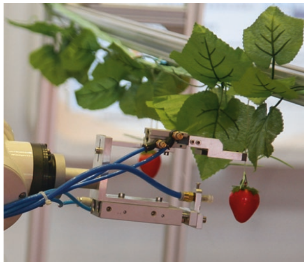
Fig. 8.9 An end-effector with air suction as auxiliary clamping unit designed for picking strawberries (Feng et al. 2012)
