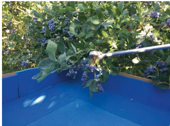
Fig. 16.3 An example of using mechanical harvester to vibrate blueberries in bushy architecture in a commercial orchard in Washington State, USA (Image Courtesy of Dr. Long He)
