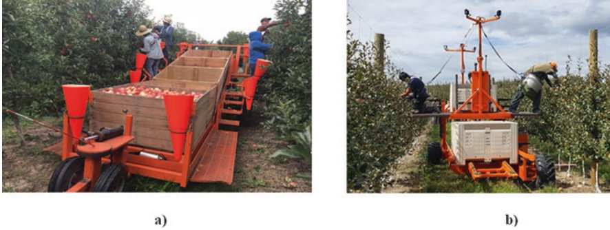
Fig. 11.1 Two commercial apple harvest platforms with no bin filler, on which workers still need to carry picking buckets for holding picked apples temporarily, until the buckets are full and dumped to the bins
