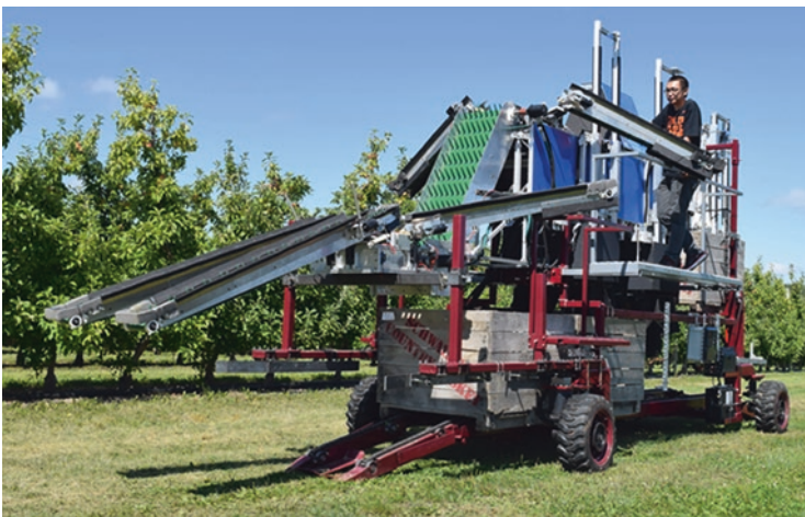
Fig. 11.5 Apple harvest and infield sorting machine being tested in a commercial orchard in Michigan during the 2017 harvest season
