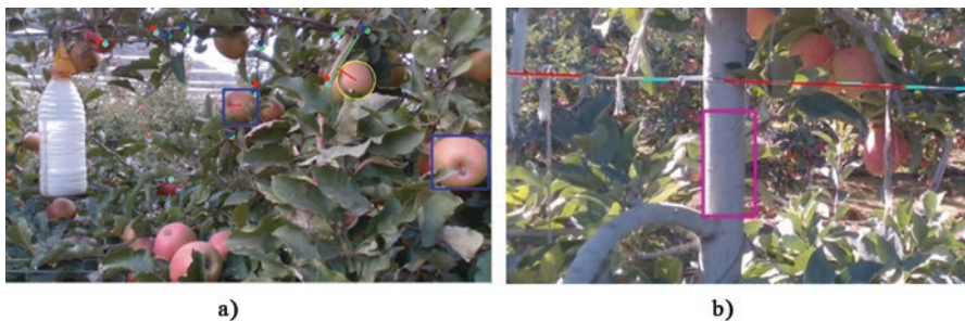
Fig. 3.16 (a) Apples marked in the image are identified and located to be safe to harvest in the given view; (b) Trellis wire and trunk detection and localization to avoid end-effector and trellis wire collision
