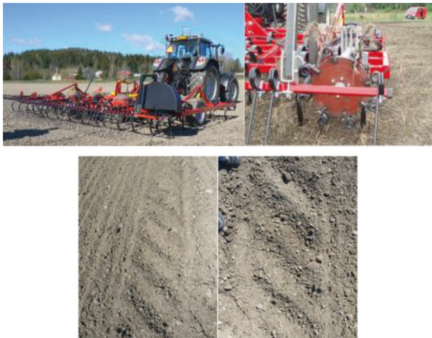
Fig. 10.5 A harrow with marker device that created improved feature to be detected with higher confidence with machine vision. (Image: Timo OKSANEN)
