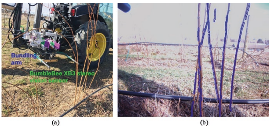
Fig. 3.19 Robotic cane bundling machine for red raspberries based on a stereo vision system (a) and raspberry canes detected and separated using 2D and 3D image-processing techniques (b). (From Bhusal et al. 2018)
