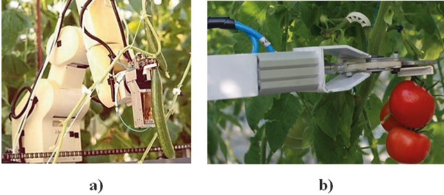
Fig. 8.11 Various end-effectors designed to hold and cut fruit stems: (a) a cucumber picking end-effector (from Henten et al. 2002); (b) a tomato picking end-effector (from Feng et al. 2018)
