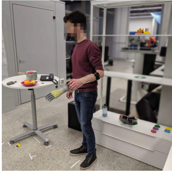
Fig. 1 The experiment setup included a Myo armband for sEMG, an i-LIMB revolution prosthetic hand, a computer, and several household objects
