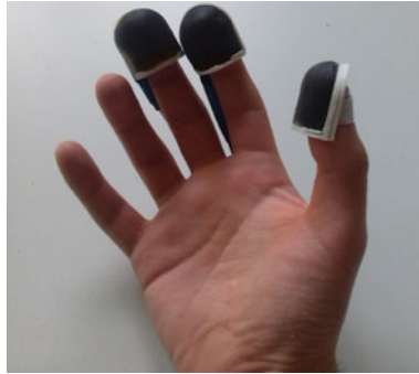
Fig. 1 The wearable sensorised thimble for grasping rehabilitation. Three prototypes for thumb, index and middle finger have been manufactured
