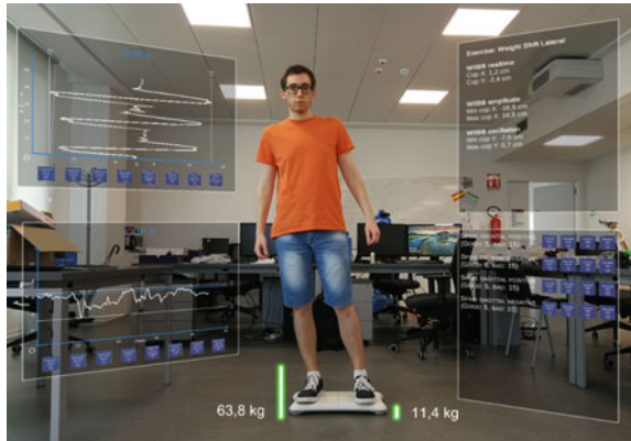
Fig. 1 View of what the therapist sees through Hololens. Around the patient, metrics describing his/her performance are shown. On the left side, it is possible to see the progress of COP over time, while on the right, summary metrics and monitoring parameters can be found
