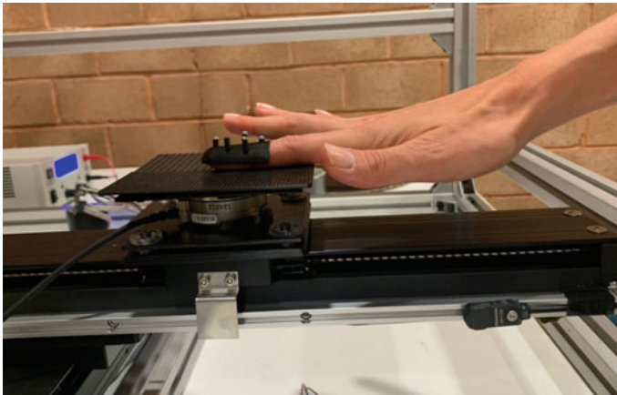
Fig. 1 The HaptiTrack device fixed inside a safety cage with mounted OptiTrack Flex13 cameras in each corner
