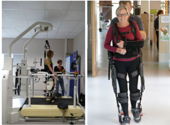
Fig. 1 Illustration of a person in the static Lokomat (left) and dynamic Ekso GT™ (right) exoskeleton (© Johan Swinnen)
