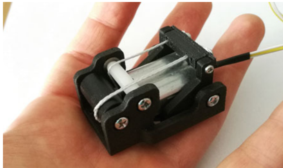
Fig. 1 Prototype of the developed parallel actuated haptic device (held in a hand for size comparison)
