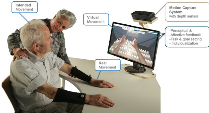
Fig. 1 The RGS setup illustrating its different components and underlying hypotheses
