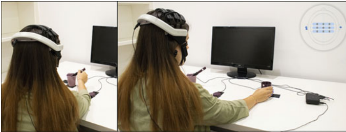
Fig. 1 Wireless dry-EEG device during the execution of the reach-and-grasp actions
