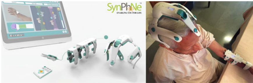
Fig. 1 The SynPhNe device with electroencephalography (EEG) and electromyography (EMG) sensors and software user interface
