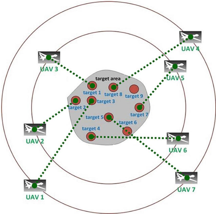
**Fig. 1** An example scenario with seven UAVs and nine targets. The UAVs have fixed flight paths, which follow one of two circular paths around the area containing the targets that are candidates for surveillance
