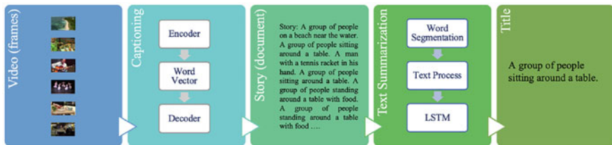
Fig. 2 This is the overall architecture of the proposed method that parts to two separate process for the video captioning and text summarization
