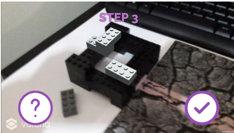
Fig. 2.7 Coop AR’s augmented reality view, where the apprentice/visitor can see the physical piece and explore it using a set of instructions. In this example, the physical lego are augmented with virtual legos
