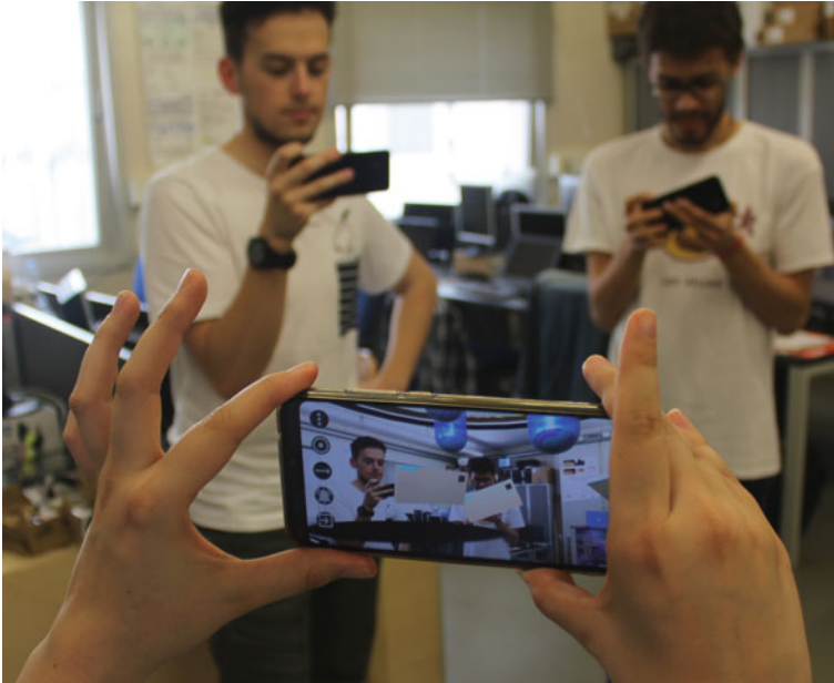
Fig. 2.9 Multiple augmented reality users sharing the same scenario and referential. Note how the system identifies each unique user in their real-life position
