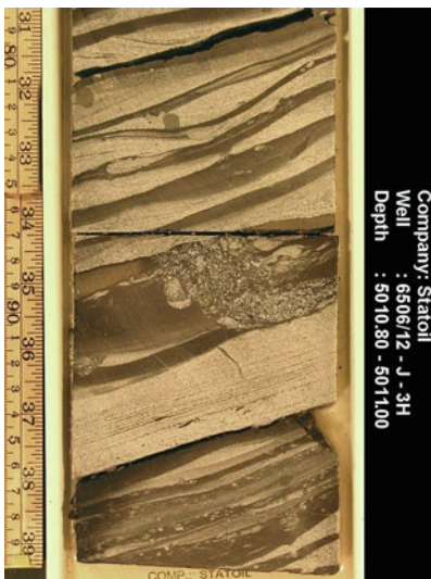
Fig. 6.16 Example tidal heterolithic facies from core – in this case an inter-tidal wavy-bedded unit showing flow ripples and some bioturbation. (Photo A. Martinus/Equinor © Equinor ASA, reproduced with permission)
