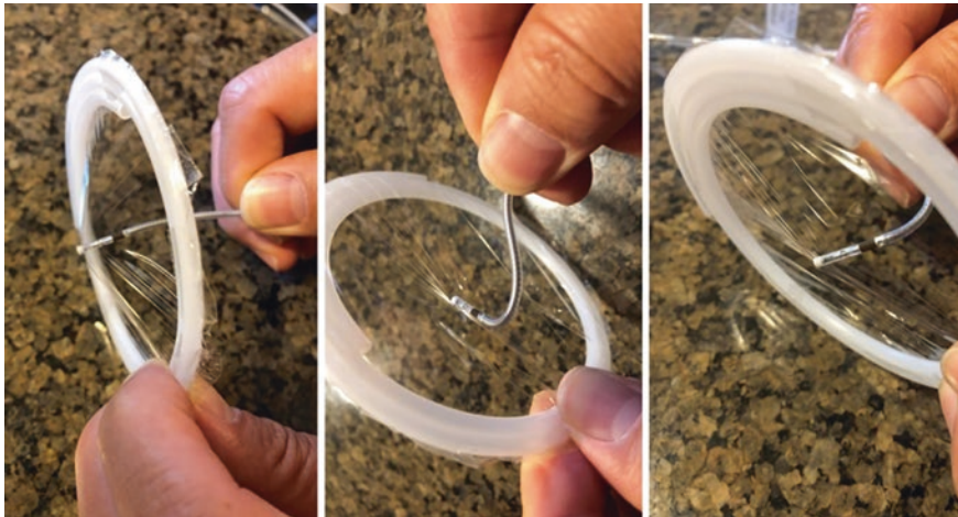
Fig. 9 The tip of ICD lead with and without stylet. (The tip of ICD lead is very stiff when the stylet is advanced all the way in. All tension is delivered to the tip of the lead and the transparent cellophane can be perforated easily (left). The tip of ICD lead is relatively floppy if a stylet is in the middle of the lead. (middle and right))
