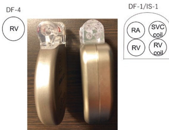
Fig. 6 ICD with DF-4 (single chamber, left) and IS-1/DF-1 (dual chamber, right) lead connector system
