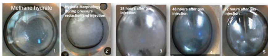
Fig. 11 Change in hydrate morphology in the presence of SDS 500 ppm in bulk water. Change in morphology is recorded before and after CO 2 injection into methane hydrate. Pictures also show the porous methane hydrate morphology. Methane hydrate formed are porous in nature (Fig. 1). Figures 2–5 shows the morphology change after CO 2 injection and 72 h after CO 2 injection [141]
