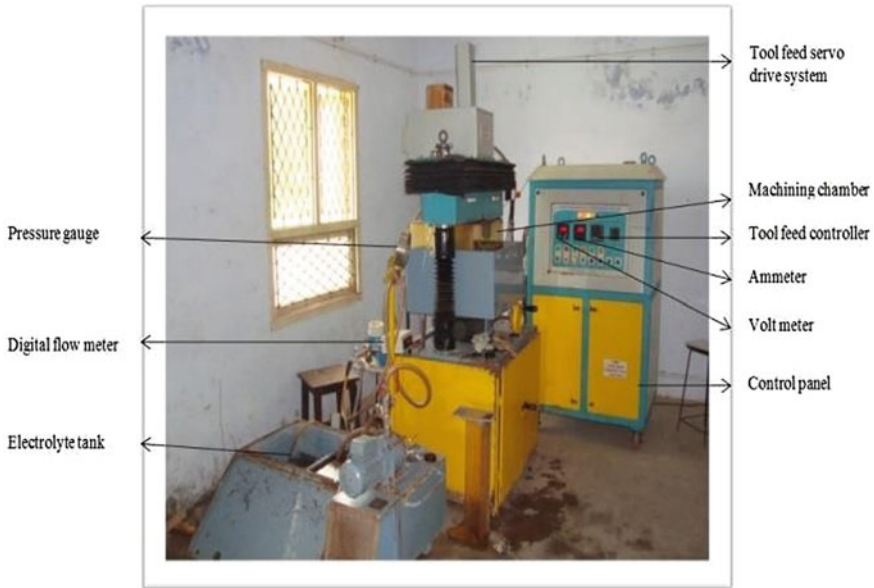
Fig. 4 Complete setup for ECM
