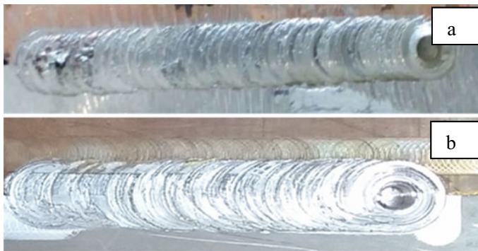
Fig. 14 Surface morphology of the weld joint a LW-WOPO at 40 mm/min, b EWW-WPO at 50 mm/min
