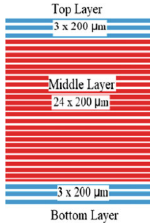
Fig. 1 Layer configuration of tensile specimen
