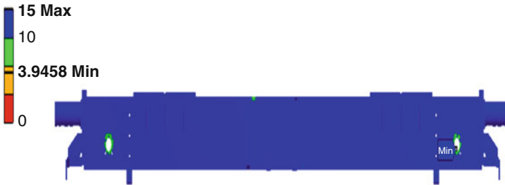
Fig. 13 Safety factor graph of x axis
