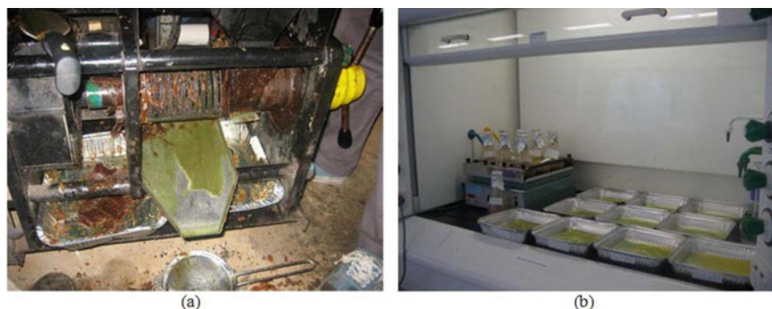
Fig. 3 Oil extraction; a Mechanical Screw Press, b chemical process [2, 3]
