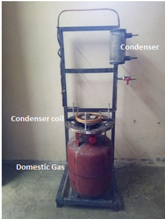
Fig. 1 Waste heat recovery model
