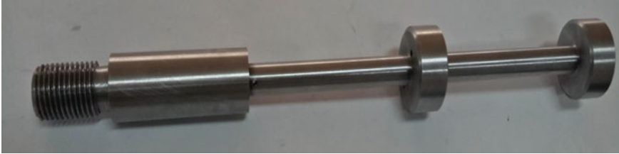
Fig. 2 The Piston rod of Omni light duty load carrying vehicle
