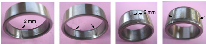
(a) One defect on outer race of N205 bearing (b) Two defects on outer race of N205 bearing (c) One defect on inner race of NU205 bearing (d) Two defects on inner race of NU205 bearing
