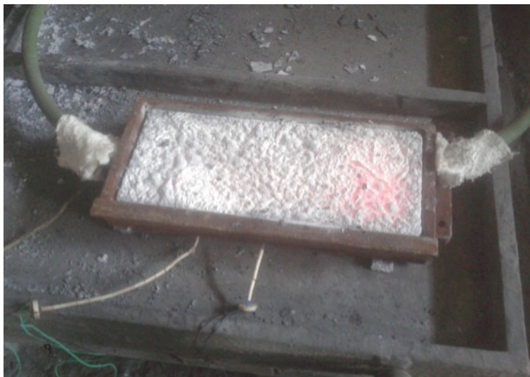
Fig. 2 Development of copper mold for 20 kg FeSiMg alloy
