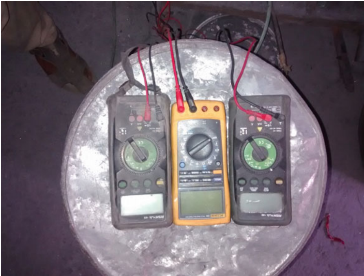
Fig. 3 Measurement of temperatures (Thermocouples)
