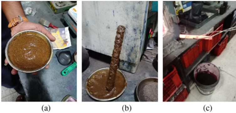
Fig. 1 a Paste b Coated Specimen and c Heated specimen
