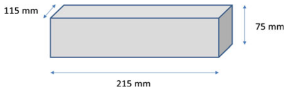
Fig. 1 Dimensions of brick mould
