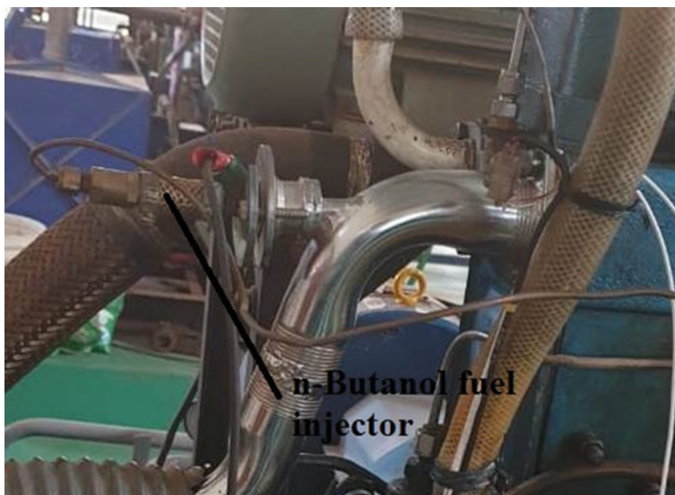
Fig. 3 n-butanol fuel injector
