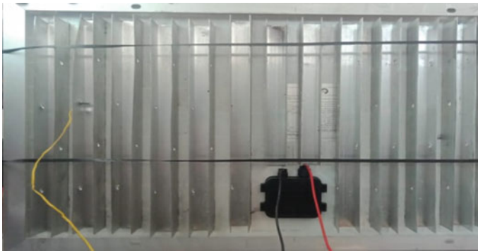
Fig. 15 14 Fin integrated experimental setup
