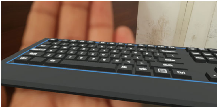
Fig. 4 Snapshot of three-dimensional virtual keyboard augmented in real-time using a mobile app
