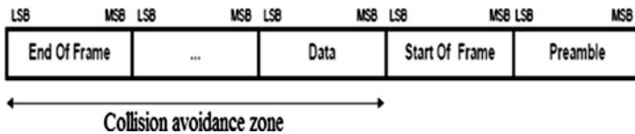
Fig. 7 Collision avoidance mechanism in Z-Wave
