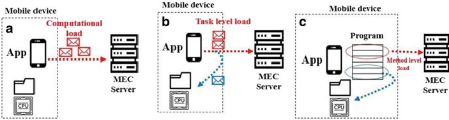
Fig. 7 Computation offloading types
