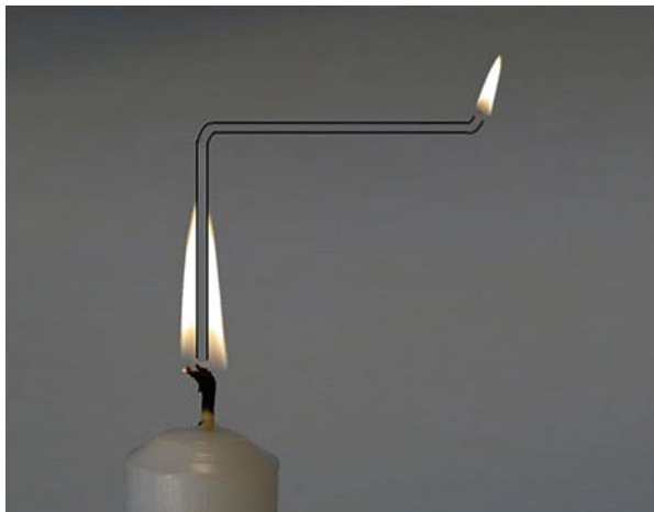
Fig. 1.2 Faraday (1861) showed the generation of flames in two different places from the vapor produced from the heated wax in a candle. One of the flames was next to the candle. The other flame was distant from the candle. The fuel passing through the tube with flammable gases from the interior of the flame only mixes with the air outside the tube where the mixture fell within the flammability limits and, provided a heat source by a match, ignited and produced flames
