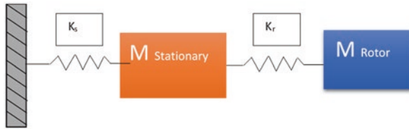
Fig. 4 Vertical motor as two degrees of freedom system
