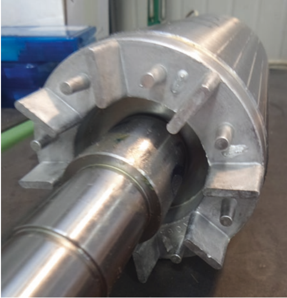
Fig. 5 View of the rotor core of the 4 kW-4pole LSSynRM prototype
