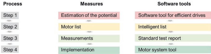
Fig. 2 The “four-step” approach developed by Topmotors, ranging from the estimation of potential through to the implementation of efficiency measures ( http://www.topmotors.ch/en/content/motor-systems-check )
