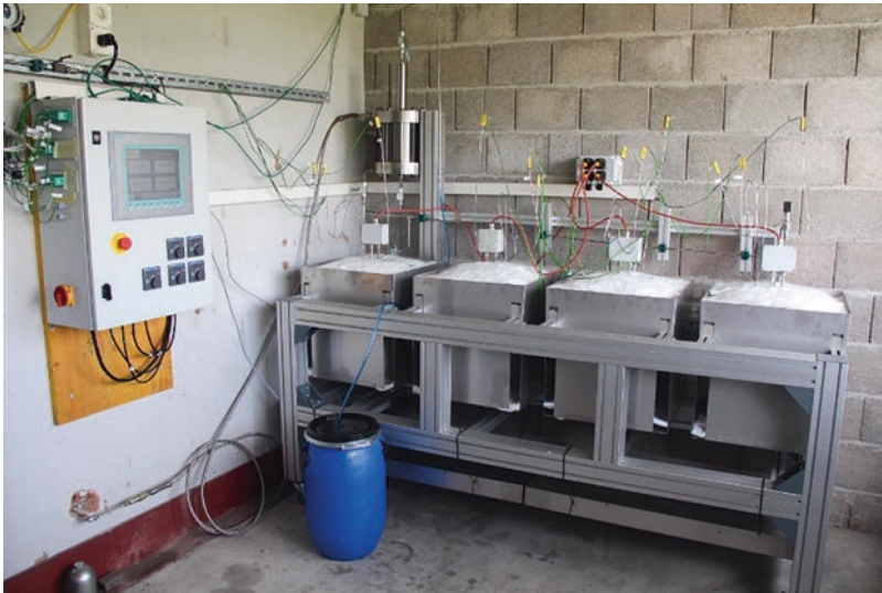
Fig. 6 Creep testing jig set-up. Four shells are simultaneously tested above 40 bar at 120 °C (248 °F), 160 °C (320 °F), 180 °C (356 °F), and 204 °C (399 °F) for 10,000 h
