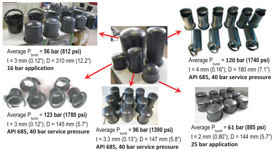
Fig. 3 Room temperature burst pressures of different shell sizes and geometries
