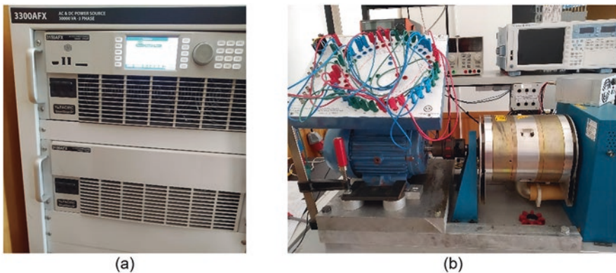
Fig. 1 Experimental setup: (a) programmable power source (AFX3300); (b) induction motor with reconfigurable stator windings mechanically coupled with a hysteresis brake
