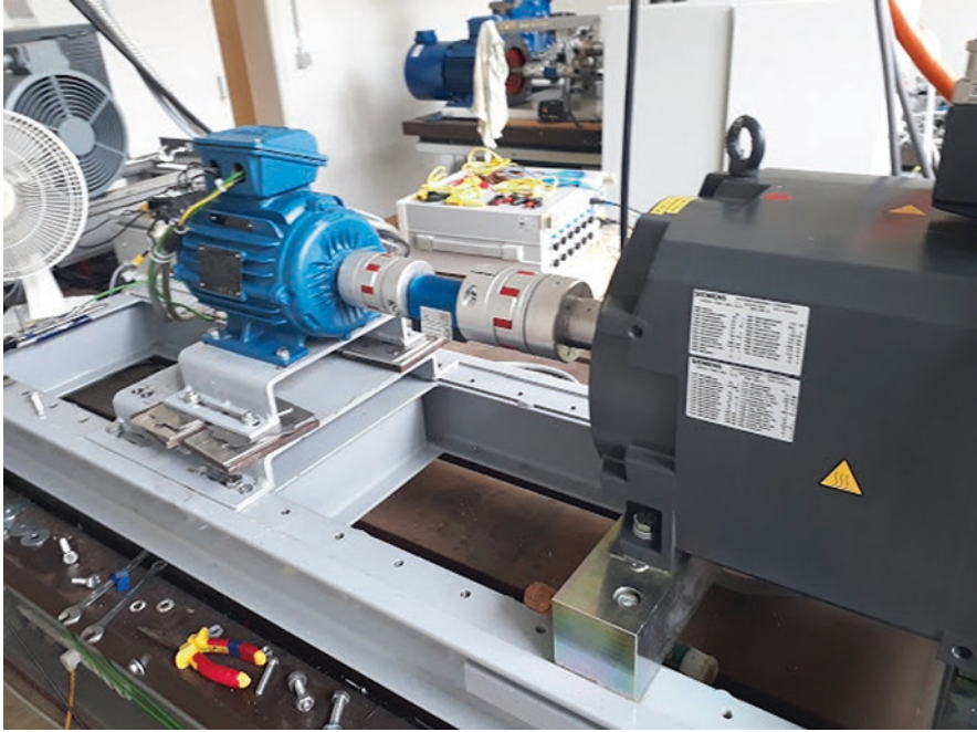
Fig. 10 Test bench with EC-motor loaded by a PMSM machine emulating a fan application
