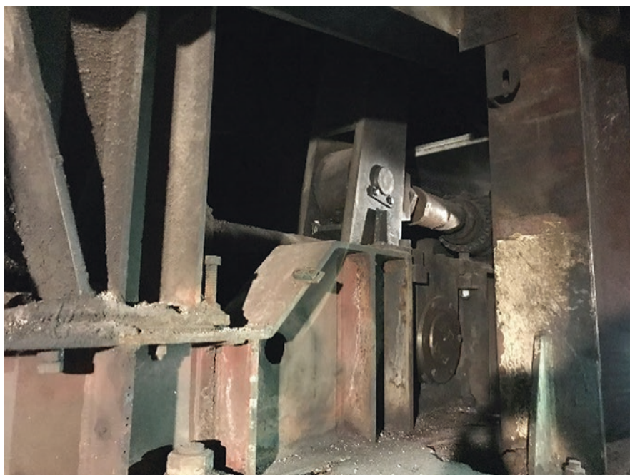
Fig. 10 Cylinder for the horizontal movement
