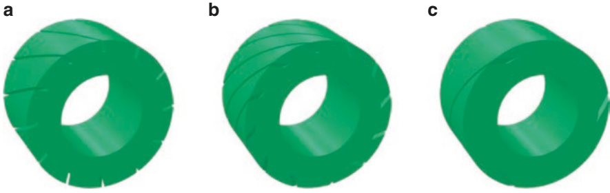
Fig. 4 Design of the rotor geometry for the skewed slots. (a) 22.5° skewing (b) 45° skewing with overlapping (c) 53.5° skewing without overlapping
