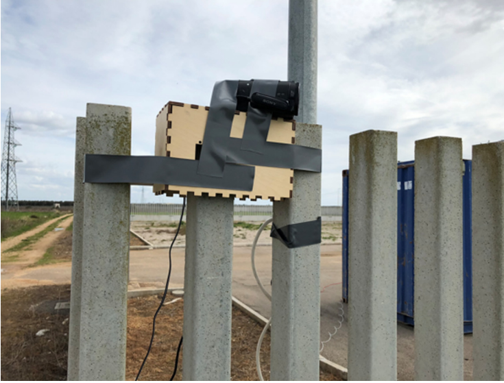
Fig. 4. Detector installation for intruder detection
