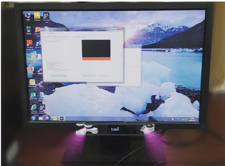
Fig. 1 Eye-tracker setup of the experiment
