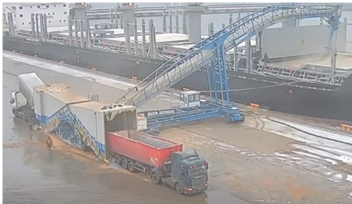
Fig. 1 Overloading of grain cargoes from trucks to ship using mobile loading mechanism
