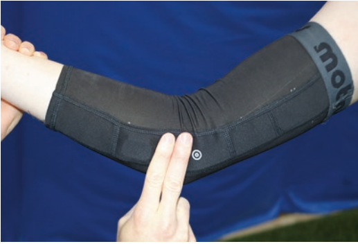
Fig. 4.1 IMU within athletic compression sleeve and positioned distal to the medial epicondyle
