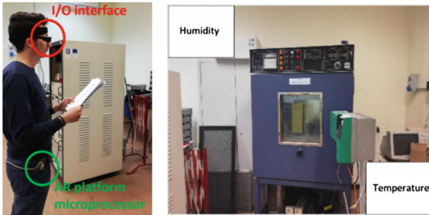
Fig. 2 On the left, picture of a User wearing AR glasses and the BCI. On the right, picture of what the User sees through the AR glasses. The writings “Humidity” and “Temperature” flicker at different frequencies [4]
