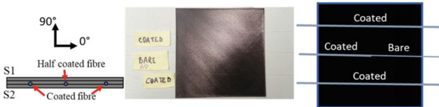
Fig. 2 Specimen A details; a scheme of the fibre type and positioning through the thickness, b photo of S1 surface, c scheme of the specimen plan view with fibres details and positioning
