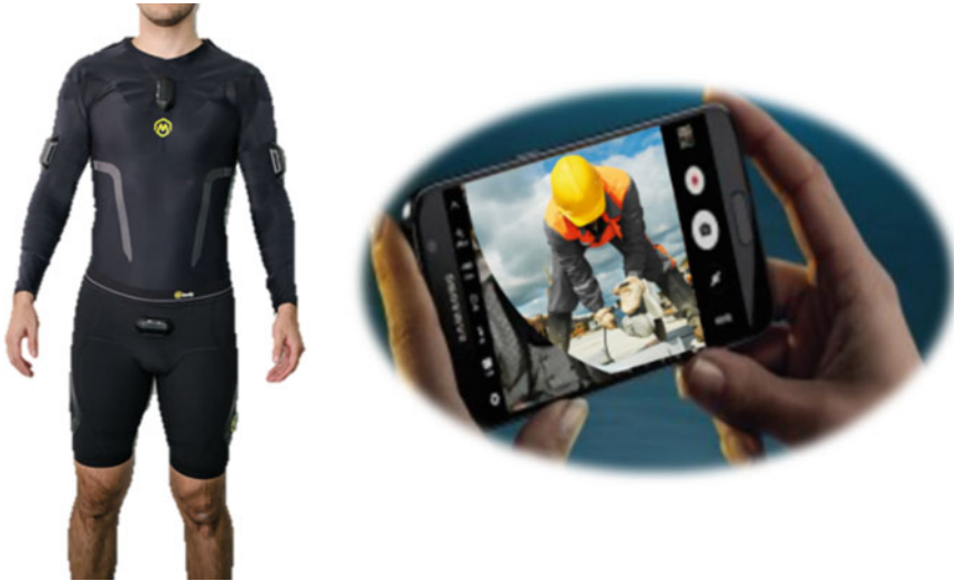
Fig. 1 The ErgoAnalysis™ System comprising of Smart clothes with sensory and mobile app controlling the system and recording video during the work
