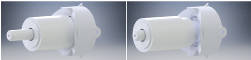
Fig. 1 The wrist design—locked (left) and unlocked mode (right)
