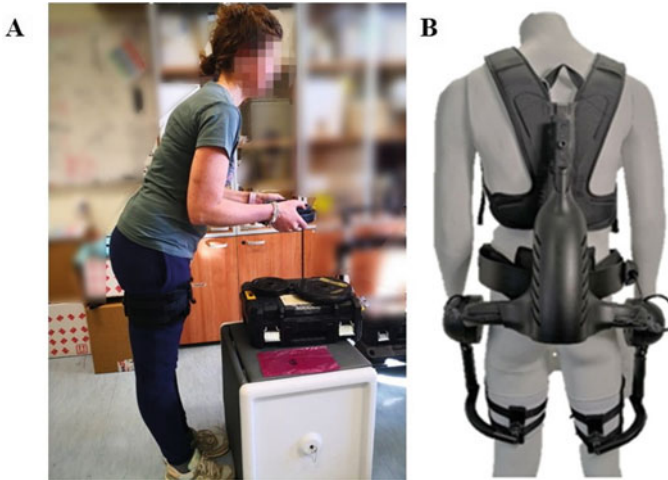
Fig. 1 Panel A: an example of the experiment with a subject holding the load with a trunk bending of about 30° in the no Exo condition. Panel B: the exoskeleton used for the experiments
