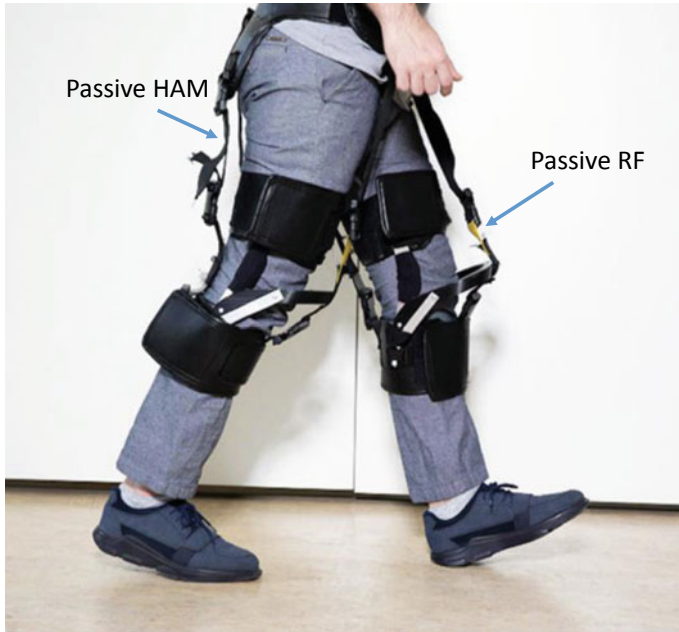
Fig. 1 Soft passive exosuit from Lauflabor. Parallel elastic elements: RF = rectus femoris, HAM = hamstrings
