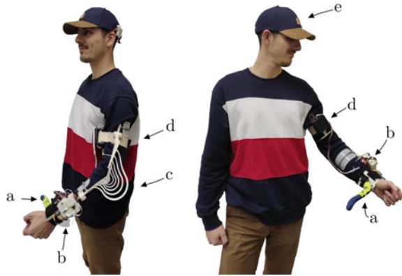
Fig. 1 The Robotic Sixth Finger (a) and its power supply and control system (b) developed by US has been integrated with the Assistive Elbow Orthosis (c) developed by UT and the CUFF (d) from UP. The CUFF has been modified to be completely wearable. Motion of the finger is controlled by a new e-Cap version (e) developed by US with novel 3D-printed electrodes by UT
