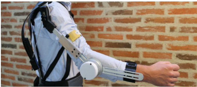
Fig. 1 A semi-active exoskeleton EXO-AIDER for upper-body motion assistance
