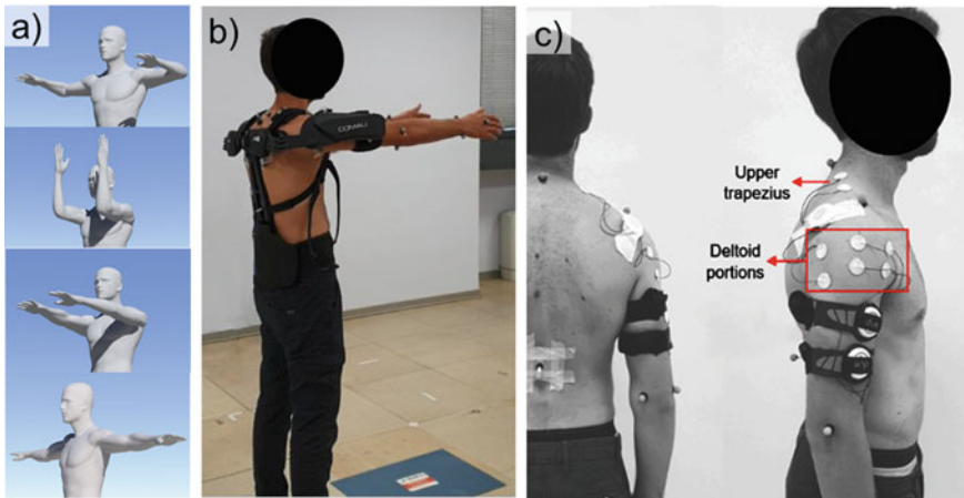
Fig. 2 a shows the four static postures considered in the study. b shows one subject wearing the MATE exoskeleton in posture P3. c The positioning of EMG electrodes
