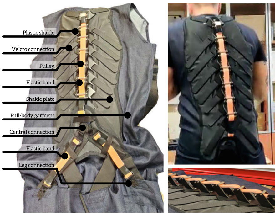
Fig. 3 FleXo prototype using the MAV mechanism. On the left, the details of the current implementation. On the top right, a user wearing the prototype. On the bottom right, a side view of the elastic band routing
