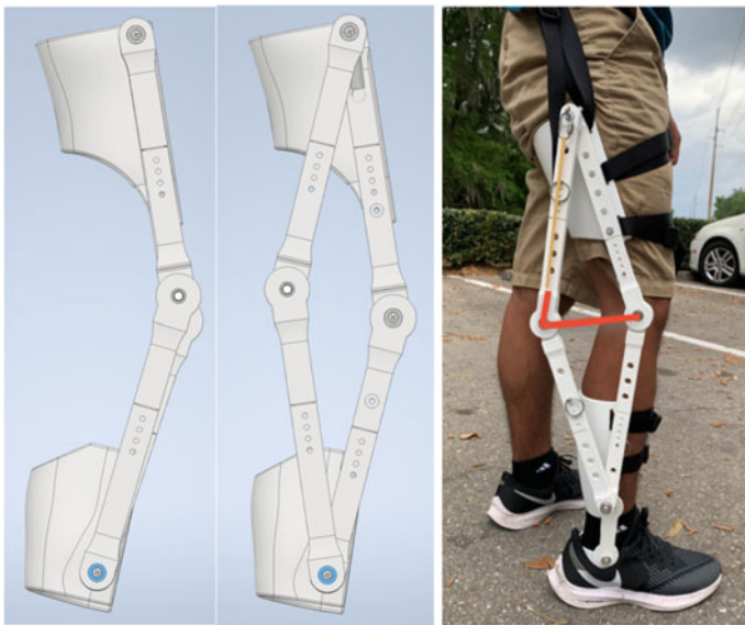
Fig. 1 Lightweight, 3D printed lower limb exoskeleton relying on elastic energy storage to assist knee extension
