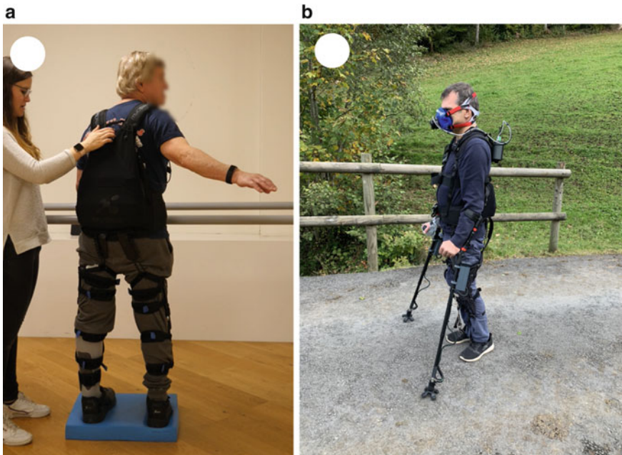
Fig. 1 The Myosuit is a lightweight tendon-driven robot suitable both for supporting its user during physical therapy (a) and to improve mobility in outdoor settings (b)
