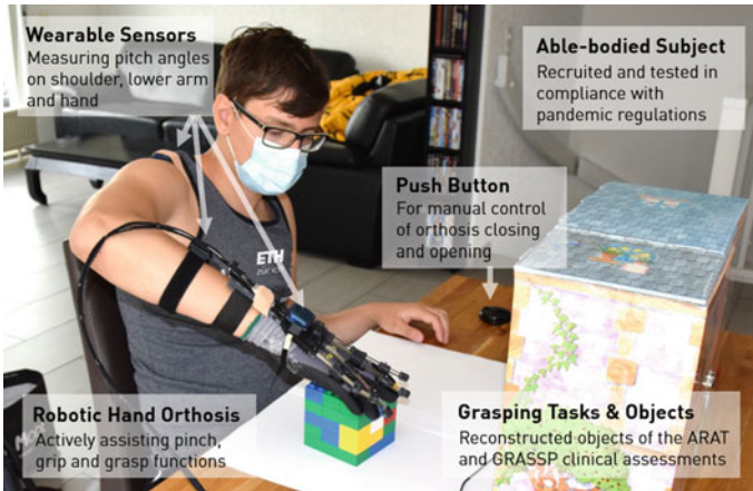
Fig. 1 Experimental setup: able-bodied subject wearing the robotic hand orthosis (RHO) and three wearable sensors (shoulder, lower arm and hand) while performing various grasp types and activities of daily living
