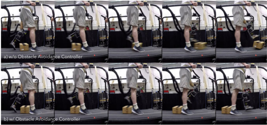
Fig. 2 User intent recognition for interactive control of obstacle avoidance. (Top) Amputee walking on the CMU powered knee-ankle prosthesis with state of art control and tripping over obstacle. (Bottom) Prosthesis control learns in real time to predict the intent of an amputee to step over an obstacle before it is encountered and helps to clear it
