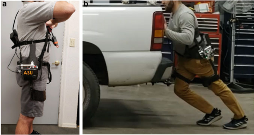
Fig. 1 The hip exoskeleton assists lifting and pushing. (Version 2 with improved thigh cuffs)
